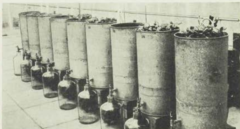
Fig. 1: The cans used in the investigation. They are shown mounted on trucks which are used to facilitate weighing to control the moisture content of the soil. The bottoms of the cans were funnel shape. A rim, attached to the sides near the bottom, served as a base.
