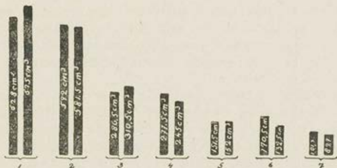
FIG. 27. — Level B of the Podsol soil. Quantities of filtrate in 21 days with distilled water and different concentrations of the \text{Ca}(\text{HCO}_3)_2 solution.
