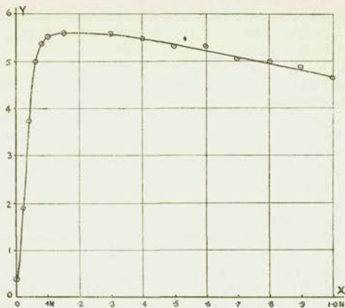
Fig. 1 "Lime-requirements" after extraction with dilute hydrochloric acid. X = Initial normality of extracting acid. Y = Millimoles of base absorbed from \text{Ca H}_2\text{CO}_3 solution per 100 g. soil.
