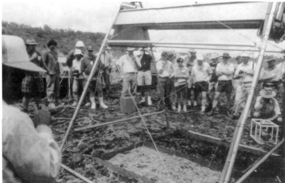
Demonstration of the portable oscillating-nozzle rainfall simulator on a vertisol with an without mulch conducted by the Queensland Department of Primary Industries research staff during the mid-week excursion.
